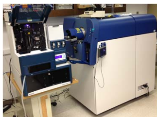
SCIEX 5600 TripleTOF with Eksigent nanoLC
